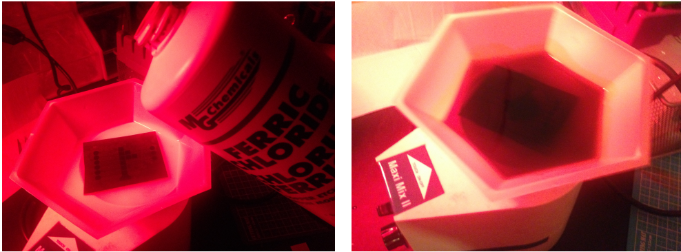
Figure 5.8. The photosensitized PCB is immersed in ferric chloride etching solution.
