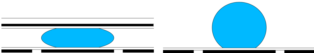
Figure 5.4. An EWOD device in sandwich (left) and open-faced (right) configurations
