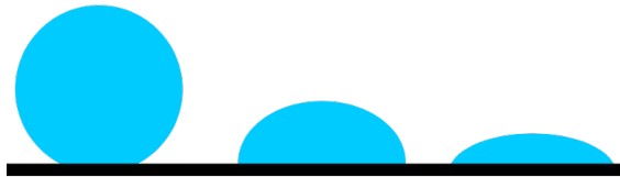
Figure 5.1. Water droplets with contact angles of (left) 120°, (middle) 90°, and (right) 50°
