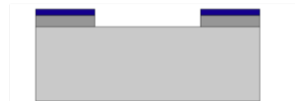
Fig. 10. DRIE through oxide layer
