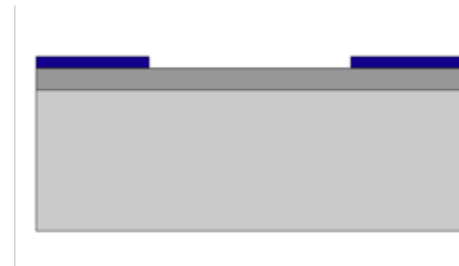
Fig. 9. Cross section of facet; exposed photoresist removed
