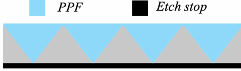
Fig. 12. PPF is deposited into negative mold
